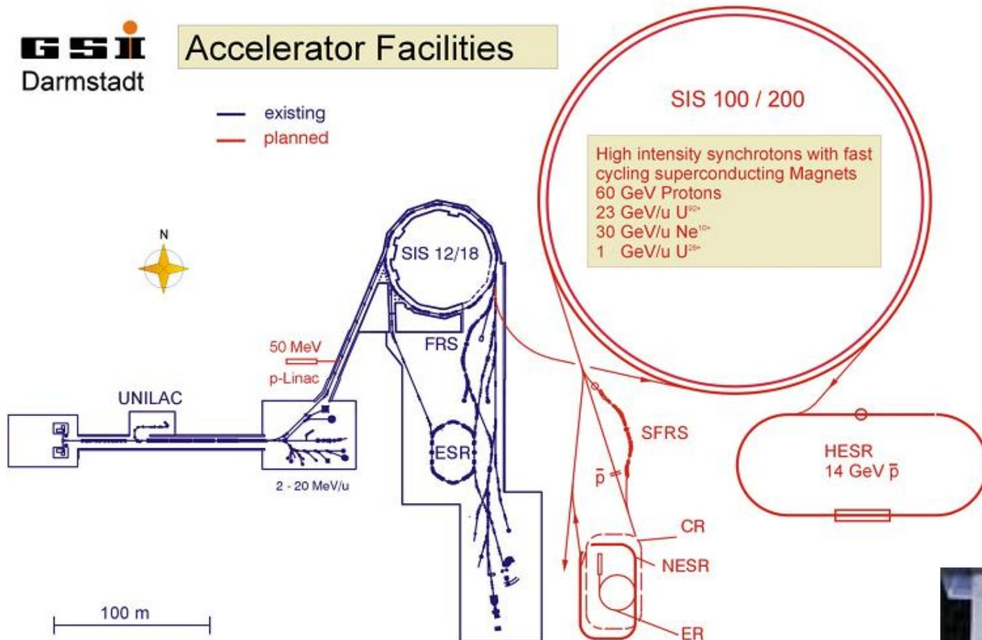
Fig.: Present Layout of the existing and planned facilities
