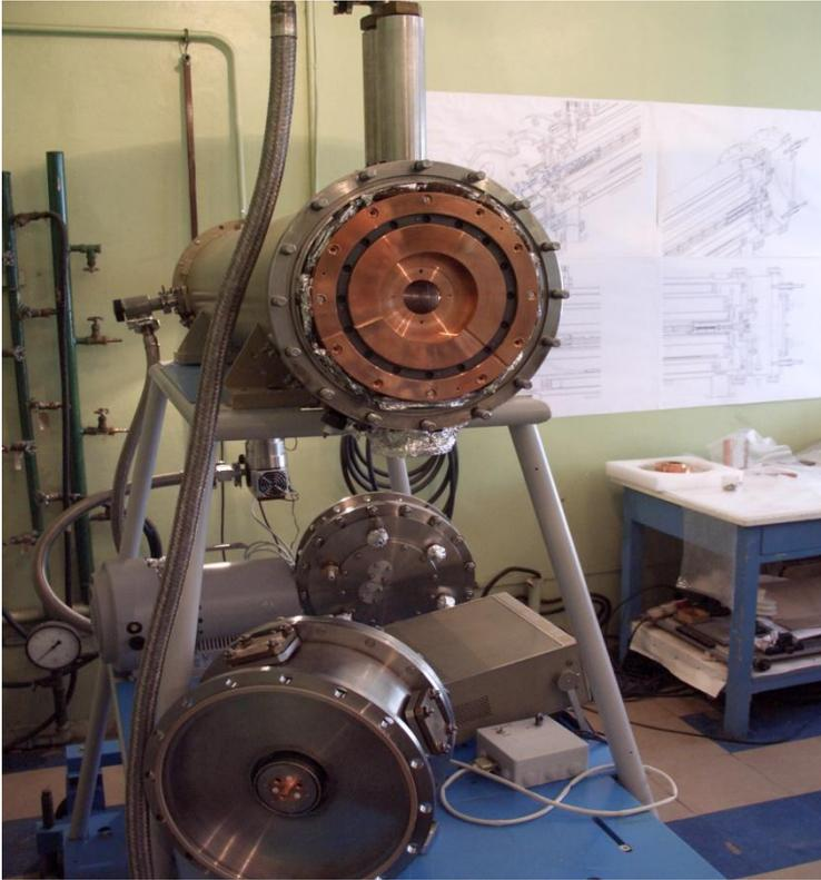
Assembling of electron/ion optics system (view from the "ion extraction" side)
