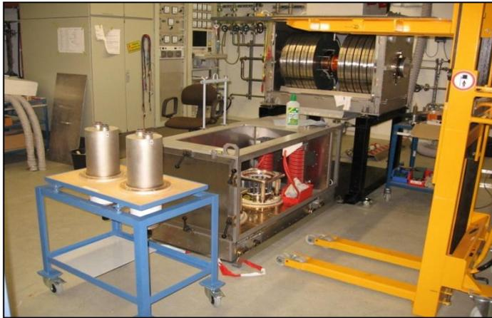
Short pulse (500  $\mu$ s), high power bunch compressor developed at GSI
