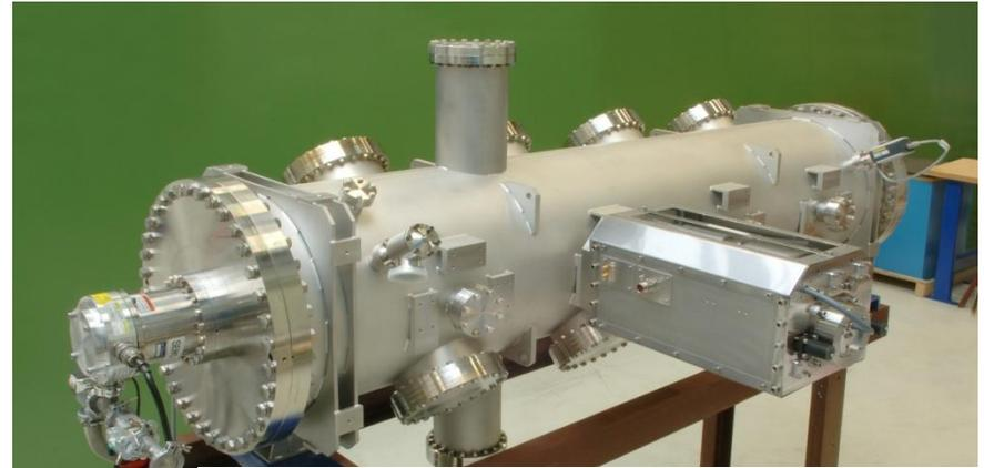
Prototype Stoch. Cooling tank with PU movers
