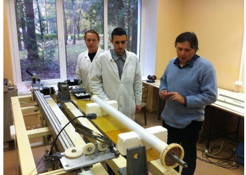
Superconducting test coil 6T
