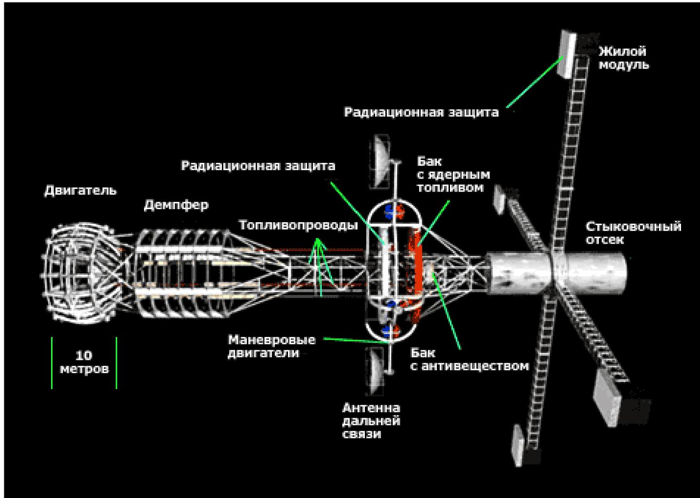
Engine is based on ACMF (Antiproton catalyzed microfission),
