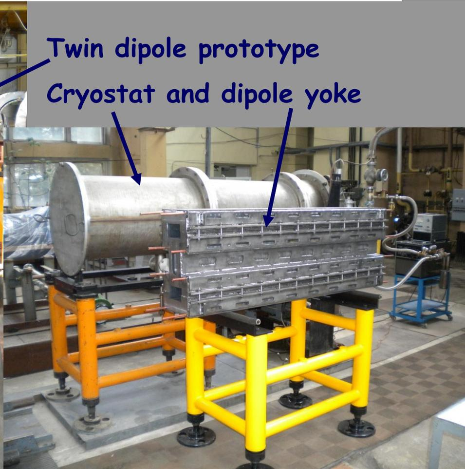
Twin dipole prototype
