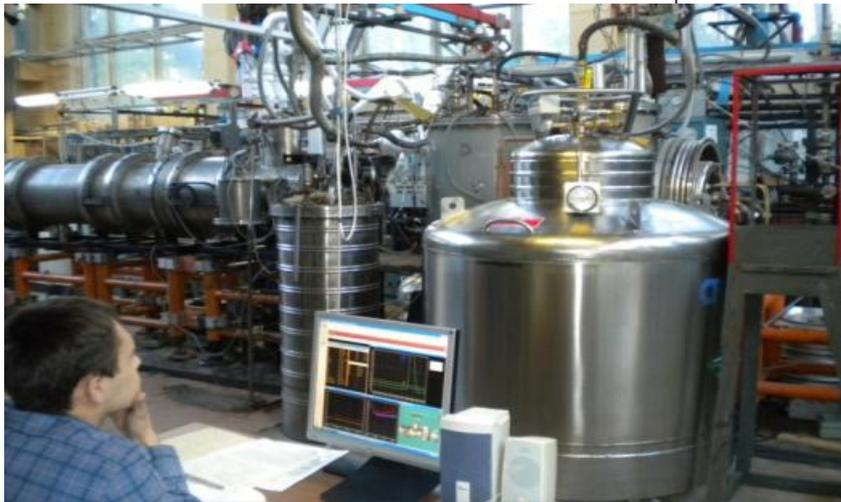
Test bench for cold tests at LHEP JINR
